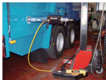
A BASH-306 powered by a hand pump used to extract corroded carriage pins of refuse collection vehicles.
